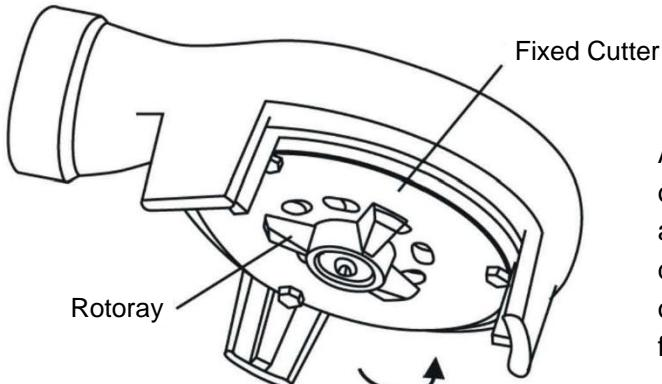
A high-speed rotating cutter is assembled at the inlet of the pump, making it easy to cut through long fibers and solid debris contained in the sewage. This design prevents the impeller from becoming blocked or entangled. This design helps prevent the impeller from becoming locked due to entanglement.
